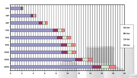
Dirt holding capacity according to ISO 16889 (test dust : ISO-MTD) of different filter media and different filtration grades. Dirt holding capacities at 2, 4, 6, 8 bar pressure difference.
